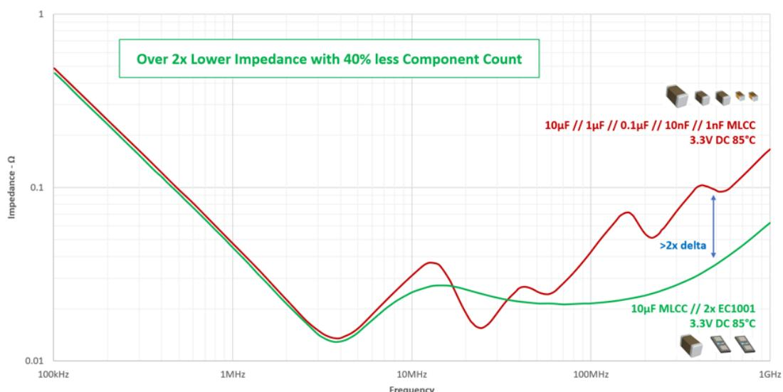
Characteristics of local de-coupling of MLCC combo vs E-CAP™
