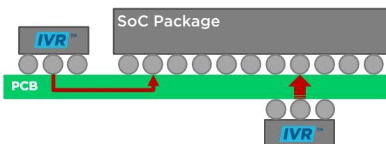
IVR™ can be mounted on back side of PCB to deliver low loss efficient vertical current to the SoC
