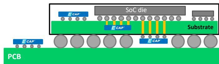
E-CAP™ can be mounted in-package for best-in-class bypass and filtering
