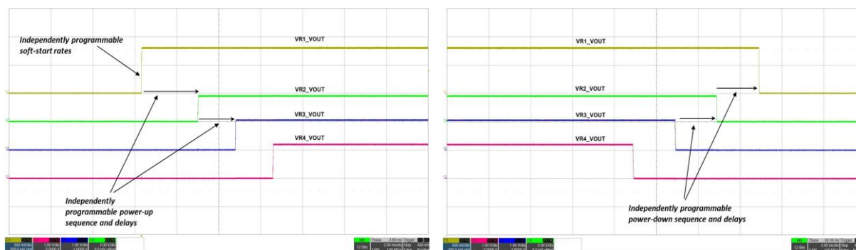
Figure 1. EP7144 Rail Sequencing: Programmable delay and power up/down of VRs
